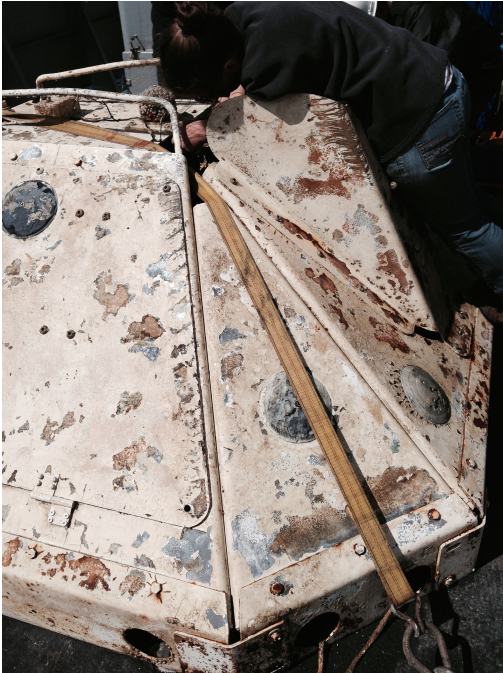
Figure 9. For the second TRM in a row, what are presumed to be trawl marks were clearly visible on the TRM recovered from FN19C . In this case the marks included deep evenly spaced gouges. Again, no evidence that the TRM had moved or of damage to the instrument itself, beyond the frame gouges.
